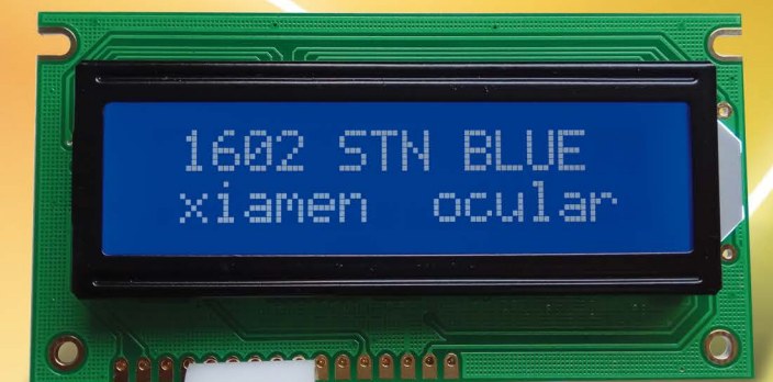
Standard character LCD modules • 4 x 1 to 40 x 4 types available • Customizable
