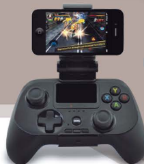
Android-based game controller with touch screen, 2.4Ghz RF or Bluetooth® optional (NS-A719)
