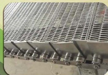
Mesh conveyor belt with guard
