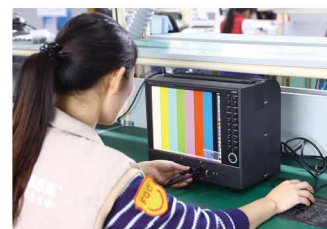
HDMI protocol analyzer for 4K x 2K @60HZ testing
